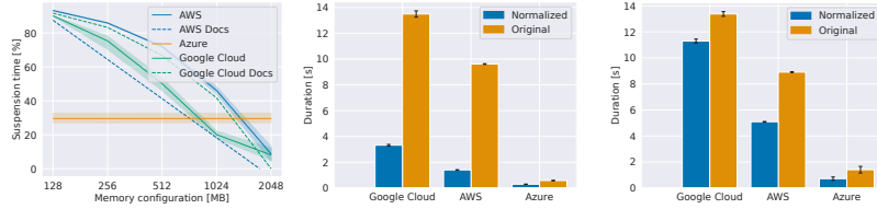
(a) Relative suspension, N = 5000 , warm . (b) Critical path of MapReduce, 256MB, burst . (c) Critical path of Machine Learning, 1024MB, burst .
