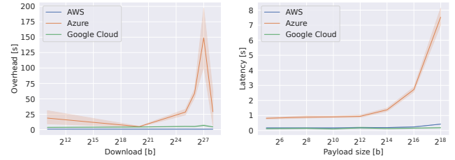
(a) Overhead of storage I/O, 20 functions, 2^{10} \leq D \leq 2^{28} , 512MB, burst invocations. (b) Invocation latency, chain of functions, 2^5 \leq M < 2^{18} , 256MB, warm invocations.
