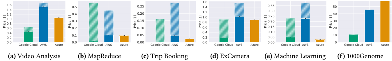
Figure 15. Price per 1000 workflow executions: function costs are opaque and state transition costs are translucent.
